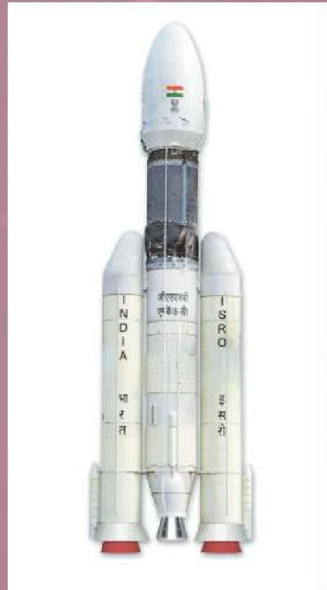
GSLV Mk III is a three-stage heavy lift launch vehicle developed by ISRO.
